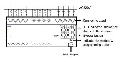
Indicator for module: Flickers when the module is working properly. Keep pressing the indicator for 3 seconds, it will turn to red, then user can read and modify the address of the module in the HDL Buspro Pro setting software.
